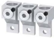
The circular conductor terminal, large, is available under separate article numbers depending on whether it is ordered with or without an auxiliary conductor terminal. With the exception of the bore for the auxiliary conductor terminal, both circular conductor terminals are technically identical, i.e. the same cable cross sections can be connected to both variants.
