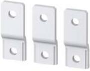
Front connection bars extended can be installed to connect larger busbars and cable lugs outside the termination area of a 3VA molded case circuit breaker. The front connection bars therefore extend the jumper lug of the breaker.
