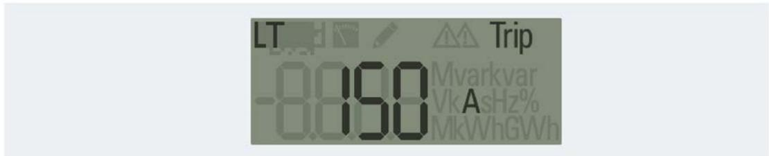
This screen can be identified by the word "Trip" which is displayed in the top, right-hand corner. The displayed current value shows the current at the moment of tripping.
