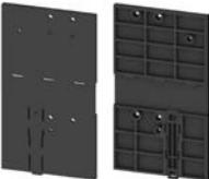
The 3VA9187-0SH20 DIN rail adapter has been specially developed for use with molded case circuit breakers combined with side mounted residual current device. This DIN rail adapter is also fitted with threaded nuts so that the molded case circuit breaker/residual current device assembly can be fastened to it by means of the screws included in the scope of supply of both devices.
