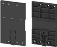
To attach 3-pole and 4-pole molded case circuit breakers to 35 mm DIN rails, a 3VA9187-0SH10 DIN rail adapter is required. This adapter is fitted with threaded nuts. The molded case circuit breakers are screwed onto the adapter by means of the fastening screws supplied with the circuit breakers. The nuts supplied with the circuit breakers are not required.
