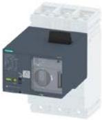
The motor operator MO320 transmits commands via electrical control cables to open and close the molded case circuit breaker. The source of commands transmitted via electrical control cables can be a pushbutton or a PLC, for example.
