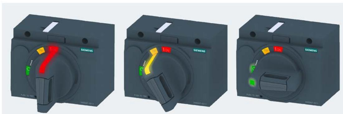
You can retrofit an active illumination kit to manual rotary operators. The illuminated indicator in the rotary handle signals the relevant switching position in the colors red, yellow and green. This provides clear visualization of the switching position on-site in conditions of poor visibility.
