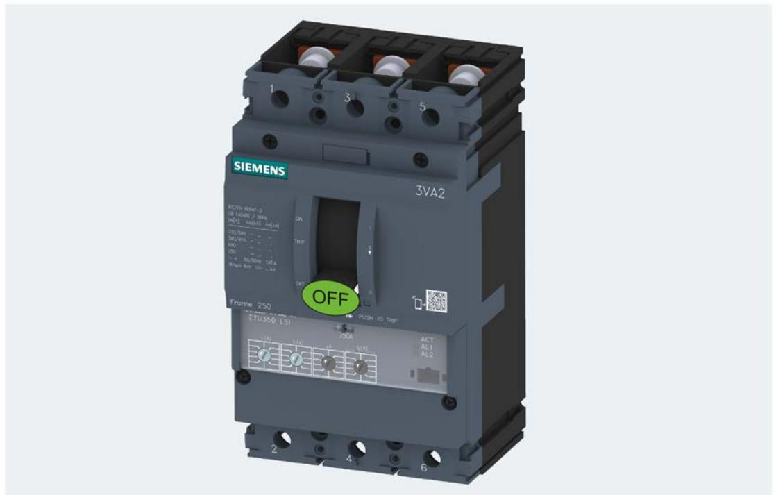
In order to prevent closure of a 3VA molded case circuit breaker, it can be locked in the OFF (O) position by a padlock. Once it is locked, the 3VA molded case circuit breaker is safely locked in the OFF (O) position. It can be unlocked again only by an authorized person.
