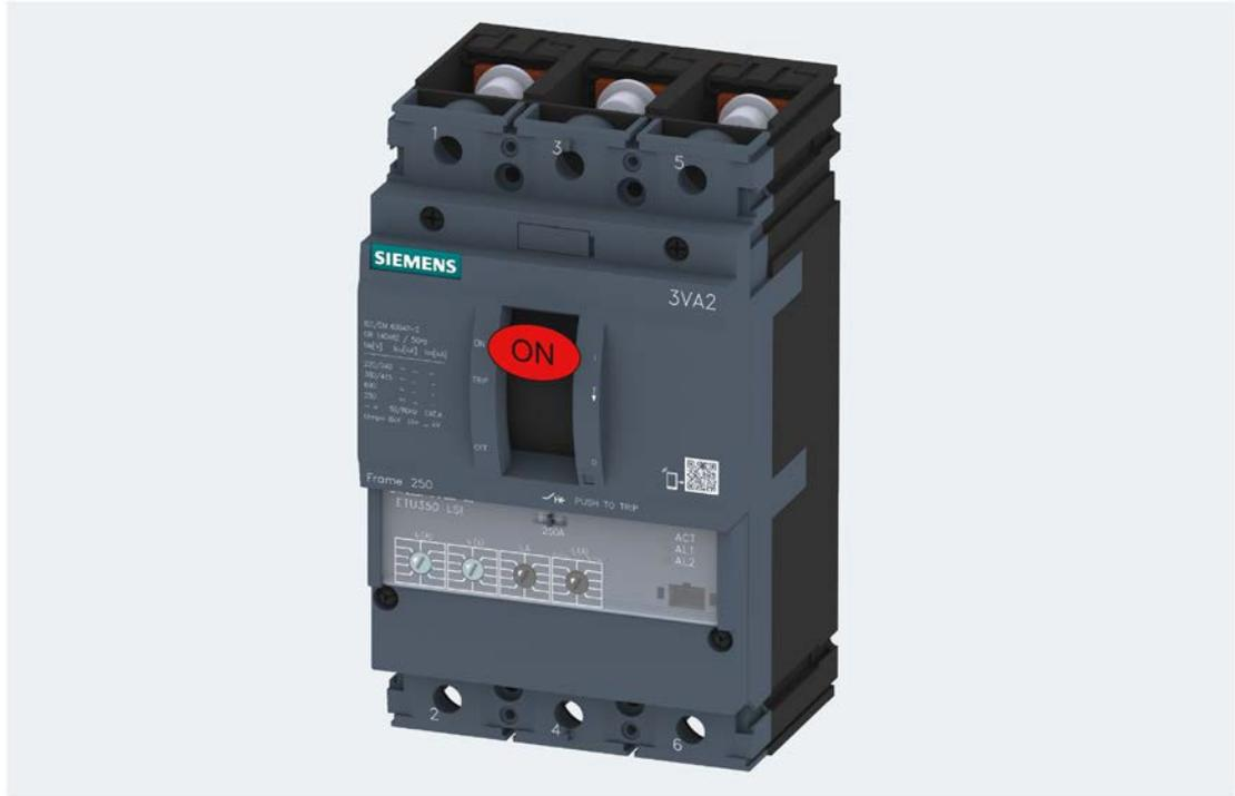
It is also possible to safely lock a 3VA molded case circuit breaker in the ON (I) position using a padlock device. The breaker contacts cannot be opened when it is locked in this position. A 3VA molded case circuit breaker can be released from its ON position again only by an authorized person.
