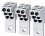
The circular conductor terminal, 6 cables is an external terminal, i.e. it projects beyond the external contour of the breaker's termination area. It can hold up to 6 cables. One of the six bores in the terminal can be used to implement an auxiliary conductor terminal.
