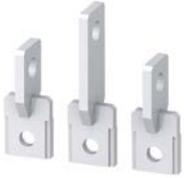
Front connection bars edgewise can be installed to connect large busbars and cable lugs outside the termination area of a 3VA molded case circuit breaker. The jumper lug of the breaker is turned by 90° when front connection bars edgewise are fitted.
