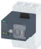
When the 3VA molded case circuit breaker is in the OFF position, it reliably disconnects all current paths of the circuit in accordance with IEC 60947-2 and IEC 60204-1 (VDE 0113). In the event of overvoltage between input and output, the reduced clearances prevent leakage currents at the surface and ensure that the dielectric strength is not degraded.
