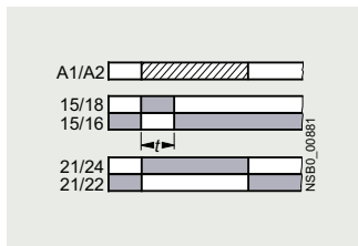
E• 3RP2005-B Passing make contact and instantaneous contact
